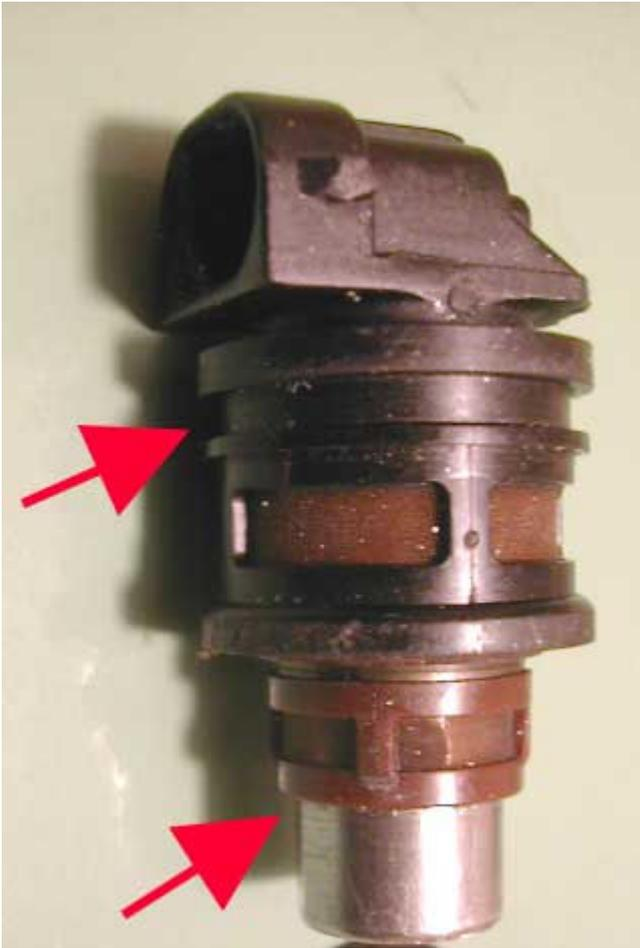
The red arrows indicate where o-rings seal against the injector. Use a little automatic transmission fluid to lubricate the o-rings. It is nearly impossible to insert the injector without lubrication.
