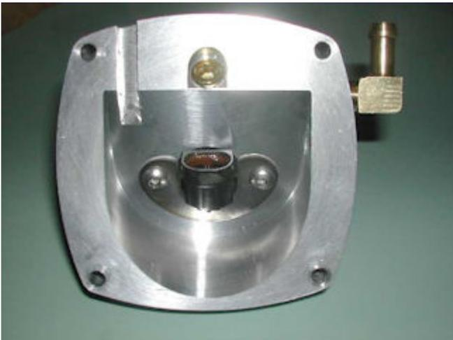
Installation of of a GM Throttle Body Injector (TBI) into the conversion insert is straight forward. This page shows the compact injector but the same principles apply to the larger bodied GM injectors. The injector pictured is the very common GM #5235277 used in 88 and 89 Chevrolet trucks.
