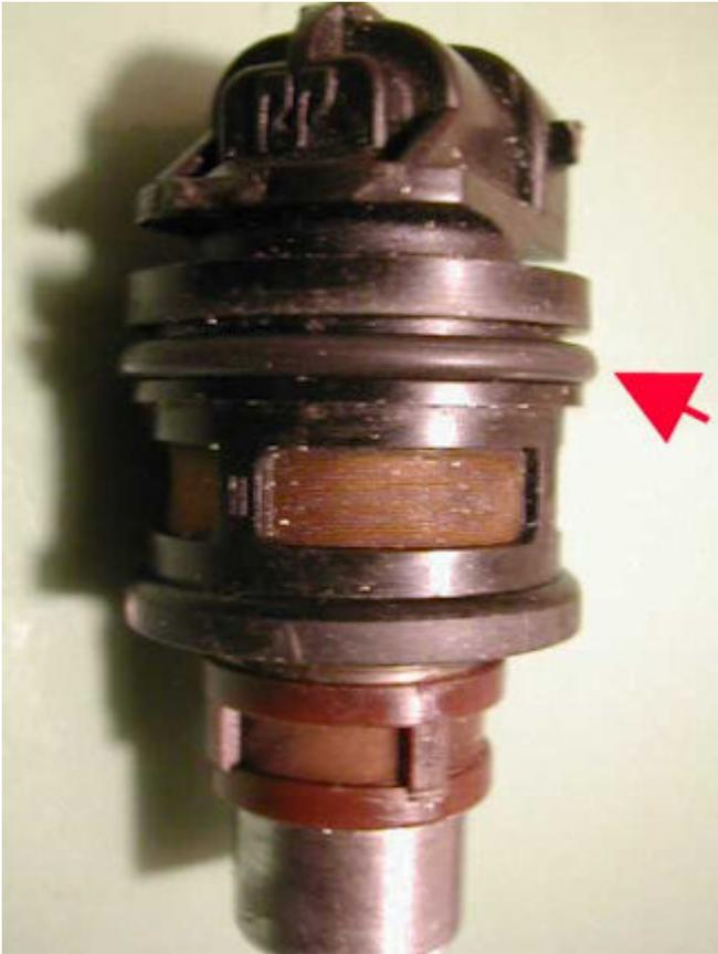
An o-ring resides in this groove and is installed onto the injector with lubrication. No sealant is used on the o-rings.
