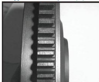
Measuring the gap between the ring gear and the shoulder on the flywheel indicated something amiss. Below: The ring gear reinstalled correctly. Photos by Jay Jablonski
