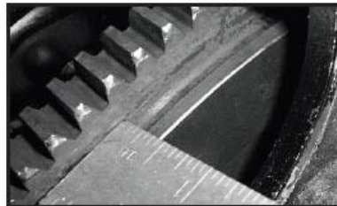
Measuring the gap between the ring gear and the shoulder on the flywheel indicated something amiss. Below: The ring gear reinstalled correctly. Photos by Jay Jablonski
