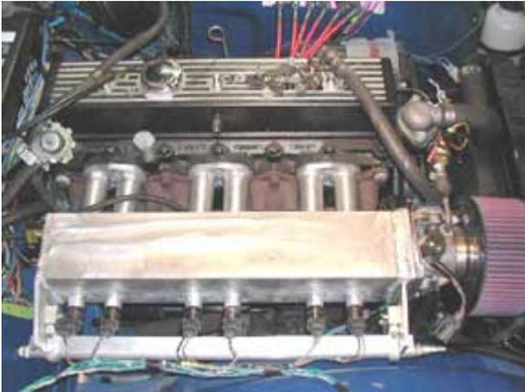
Fuel injection intake manifold with injectors trial fitting.
