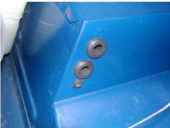
Holes were drilled and grommets added to bring the two main wiring harnesses out from under the passenger foot well. Two
