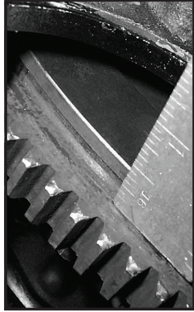
Measuring the gap between the ring gear and the shoulder on the flywheel indicated something amiss. Below:
